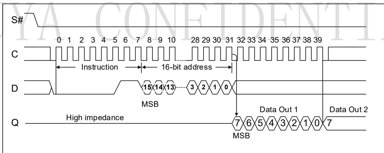
The instruction is not accepted, and is not executed, if a Write cycle is currently in progress.
