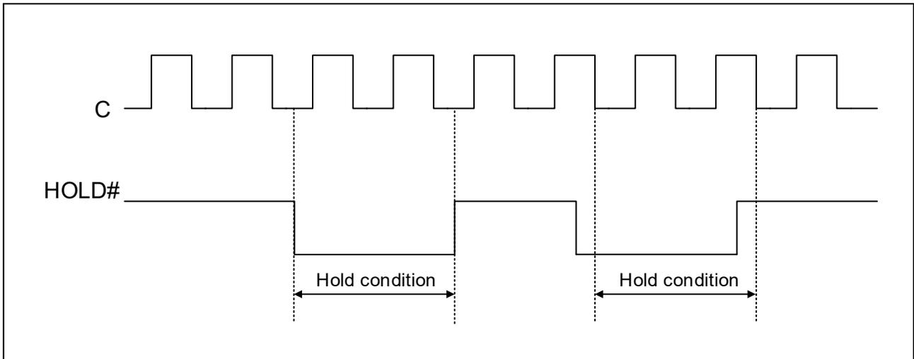
The Hold condition starts when the Hold (HOLD#) signal is driven low when Serial Clock (C) is already low (as shown in Figure 5-1).
