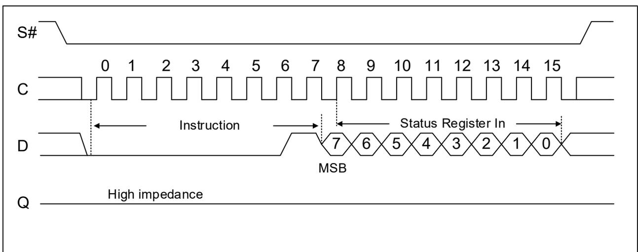
Driving the Chip Select (S#) signal high at a byte boundary of the input data triggers the self-timed Write cycle
